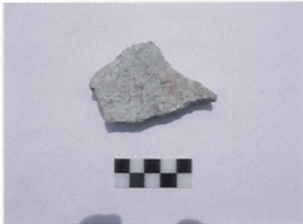
Plate 12. A mortar used to cover the adobe walls. It is a mixture of sand, lime and water.
